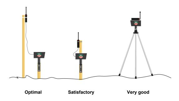
To fix the **transmitters** on wooden-post, skis or photocells, you can use Velcro, Straps, Serflex or quick fixation. Tag Heuer will be able to provide you a specific product during January 2004.
